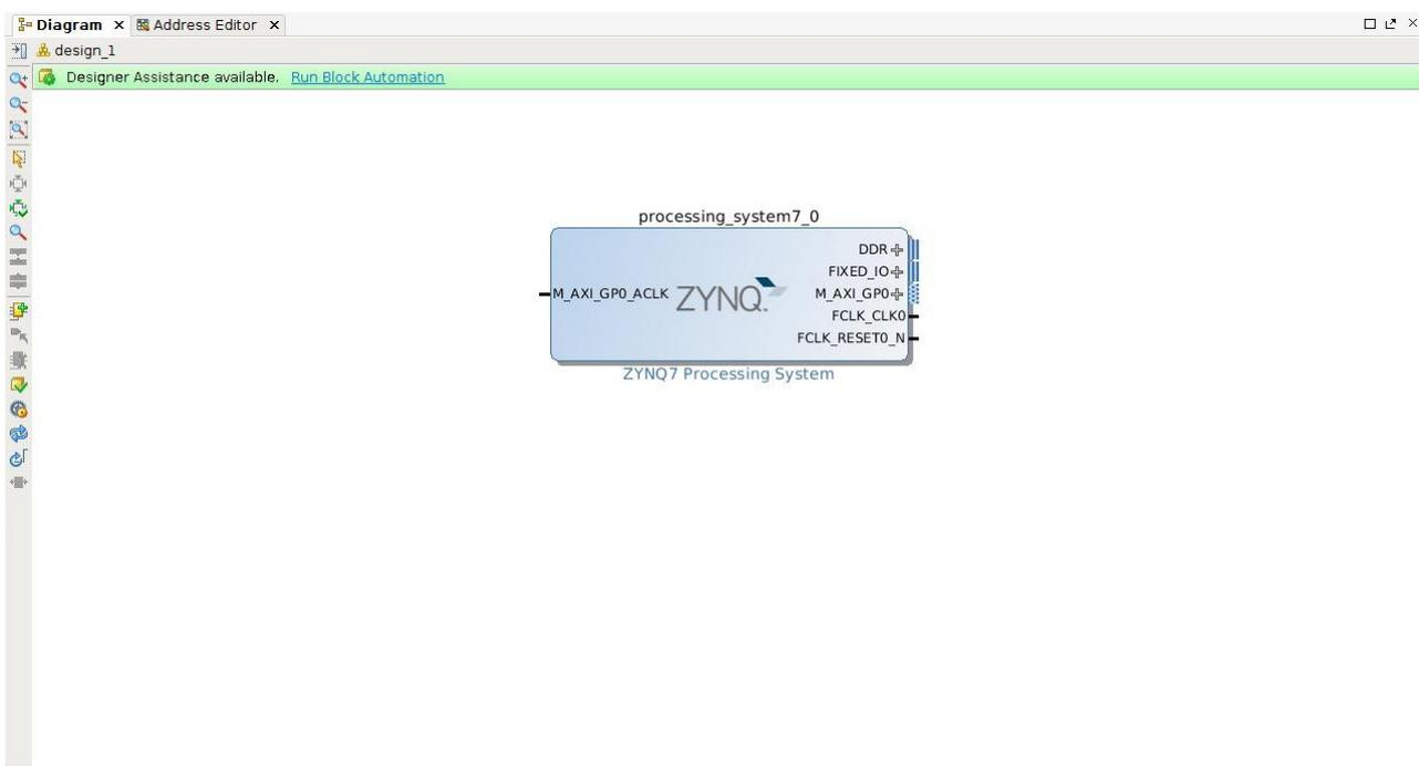
Figure 10: Vivado Block Diagram view with ZYNQ processing system.
