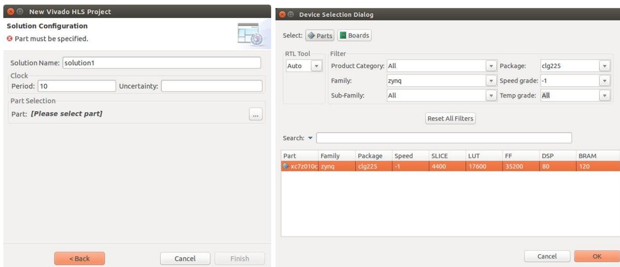
Figure 3: Solution configuration. Select the “xc7z010c1g225-1” device.
