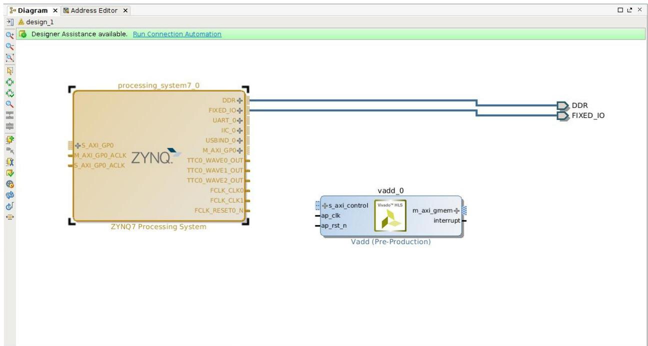
Figure 17: Block diagram view after configuration of the processing system.
