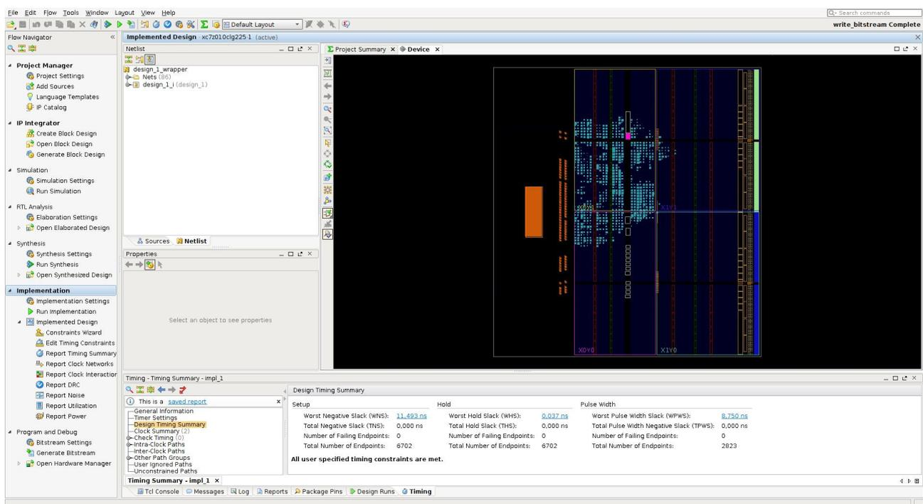
At this point we have completed the part of this guide that takes place in Vivado. The next step is to go into the file menu and select “Export Hardware” (include the bitstream) and then to “Launch SDK”.
