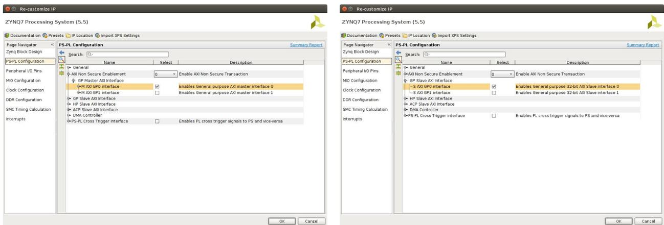
Figure 16: Configuration of the AXI Master/Slave ports.
