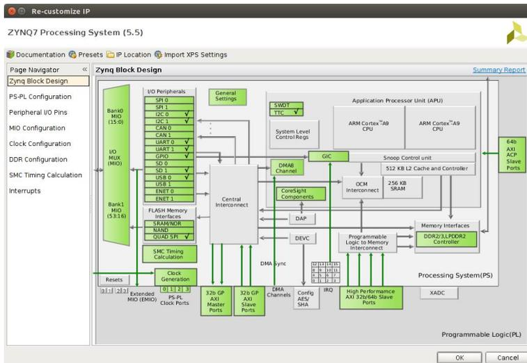
There are two interfaces that needs to be configured inside the processing system. the “32b GP AXI Master Ports” and the “32b GP AXI Slave Ports”. Double click on the Master ports and configure according to the left side of figure 16. Then do the same for the Slave ports and the right side of figure 16.
