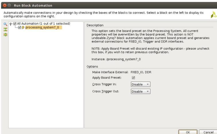
Figure 11: Block automation dialog for the Processing System.
