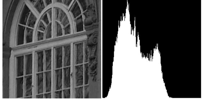
Figure 4. The right-hand image visualises the frequency with which different shades of gray occur in the left-hand one.
